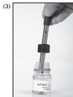
3. Plunge the sensor into the bottle of "mV465" buffer solution.
